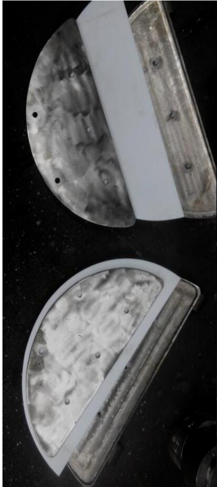
WCB+PTFE DISC(TIGHTEN BY SCREW)
